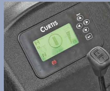
Instrument can display the steering angle and direction Synchronously
